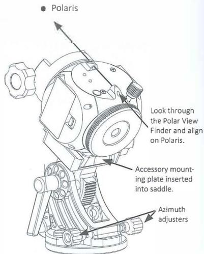
**Looking through the Polar View Finder align SAM until you can see the star Polaris in the field of view. This simple polar alignment will be adequate for most purposes.**
