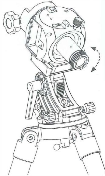
**Aim your polar scope at a distant target then rotate the Polar Scope 180 degrees so that the lock knob is on the opposite side. Next, check the position of your distant target in the eyepiece. If it has moved off centre significantly you will need to calibrate your polar scope reticule.**
