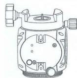
Attach to tripod via 3/8 inch base socket.
