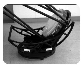
6.3 Tighten the M6x25mm Allen screws on both side of the rocker support and reinforcement bar
