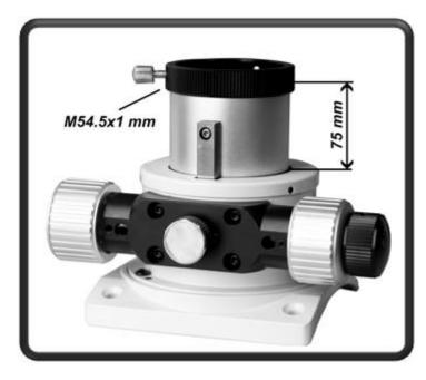
The focuser's drawtube has a maximum extension of 75mm from the base. For specific applications, requiring more than the standard 55mm back focus, it is possible to machine a custom ring (thread M54.5x1mm) to replace the 2 inch accessory support and use it as a base to affix specific accessories.
