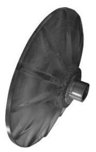
Instead of a heavy mirror blank at the standard 1:6 thickness ratios (1 cm thick for every 6 cm in diameter - so they won't flex and sag out of shape under their own weight), the StarGate 18 uses a thin composite mirror with sagittal reinforcements. This specific construction retains the same sturdiness as a standard 1:6 thickness ratio but is far less massive and will reach rapidly thermal equilibrium. The secondary flat mirror uses a cellular structure for the same purposes.
