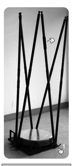
Please note that the bar with the handle grip, marked "1" should be positioned in the corresponding groove marked "1".
