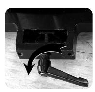
3.2 Loosen the three clamps on the rear cell to pull the cover plate open.
