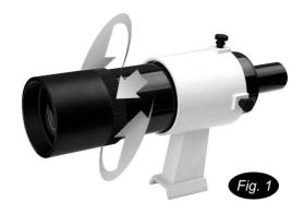
If it is necessary to refocus your finder scope, look at an object that is at least 500 meters (or yards) away. Loosen the knurled ring by unscrewing it back towards the bracket. The front lens holder can now be turned in and out of focus. When focus is reached, lock it in position with the knurled ring (Fig. 1).
