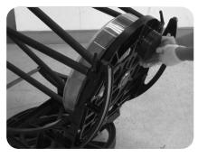
7.1 Thread the counterweight onto the M10 bolt, and then thread this bolt into the M10 hole on the back plate of rear cell.
