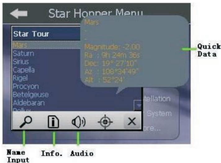
You can use the up and down keys to scroll through the selected list, or use the “Name Input” to enter the object name directly with the virtual keyboard which appears. Remember, only objects which can be seen in your current sky (based upon your time and location) will be shown on the list.
