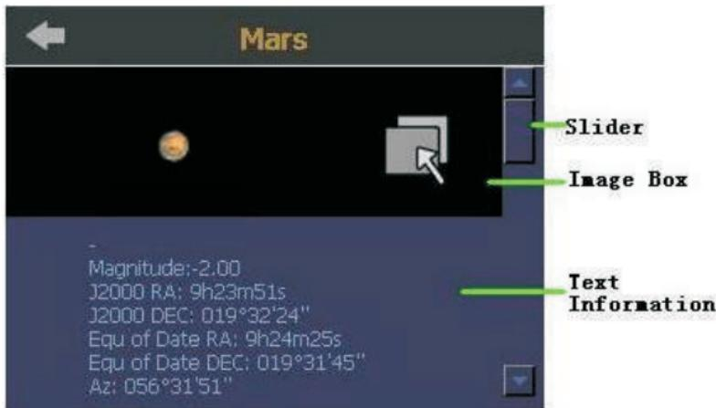
The text information zone of the window provides some basic data for the selected object. Use the onscreen slider to scroll down for more text, if it is available. If SynScan Tour has an image in its memory for the selected object, the image box will be available to select. Touching one of the “thumbnail” images within the image box onscreen will access the image. The display will now look something like this:
