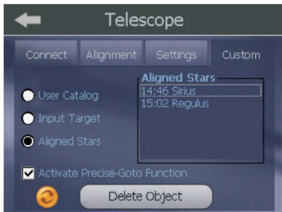
The bright stars which are used in the Precision Goto Function are recorded. Select the “Aligned Stars” circle in the Custom tab to see these stars in the “Aligned Stars” window, as shown below.
