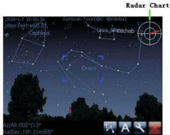
The screen then returns to the real-time sky map. It will again display the area of sky located directly behind the SynScan Tour, but now a circular “radar chart” appears in the upper right corner. There is a red line on the radar chart which directs you how to move SynScan Tour in order to point it at the selected object.
