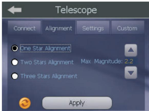
First, use the up and down buttons on the right of the touch screen to set the maximum magnitude of stars that will be used for telescope alignment. You will not usually need to adjust this, but you can set it to a lower number for a bright city sky. This will only show the very brightest stars visible from your location.
