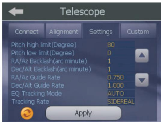
Touch a parameter onscreen, or use the Device key to choose the parameter, then use the up and down keys (or the up and down buttons onscreen) to change the value of the parameter. Use the “Apply” button to confirm the change.
